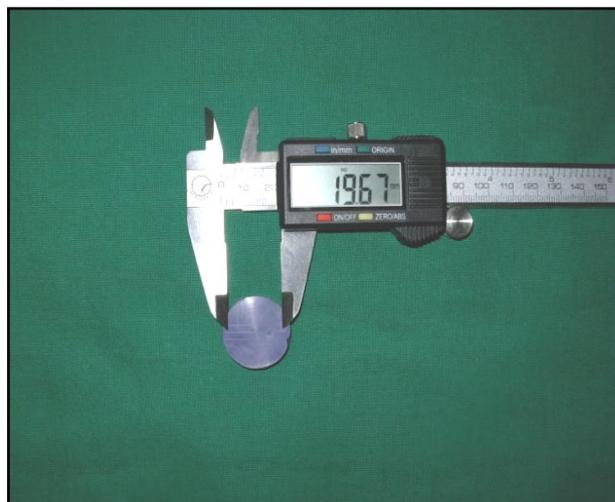
**Figure No.4:** Digital Vernier Caliper measuring the distance between lines C1 and C2 on the impression samples of polyvinyl and polyether.
