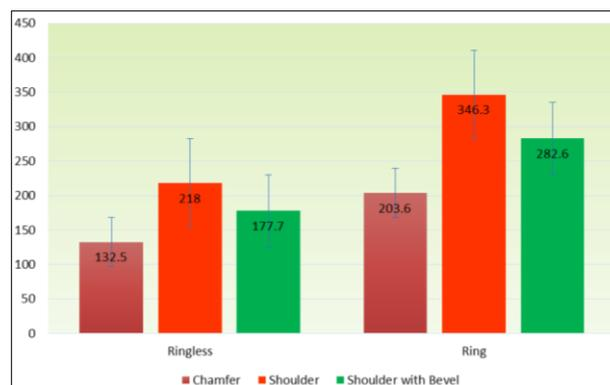
Graph 1: 2 way Anova analysis of mean marginal accuracy in vertical discrepancy of ringless and ring castings with different marginal configurations.
