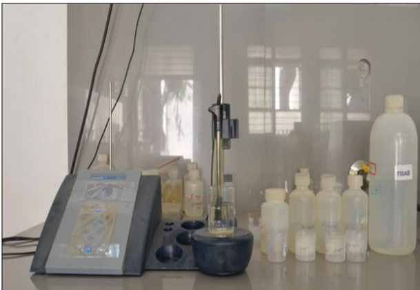
Fig 2: Specific Ion Electrode for fluoride release estimation
