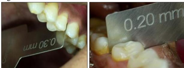
Figure 5: measurement using leaf gauge
