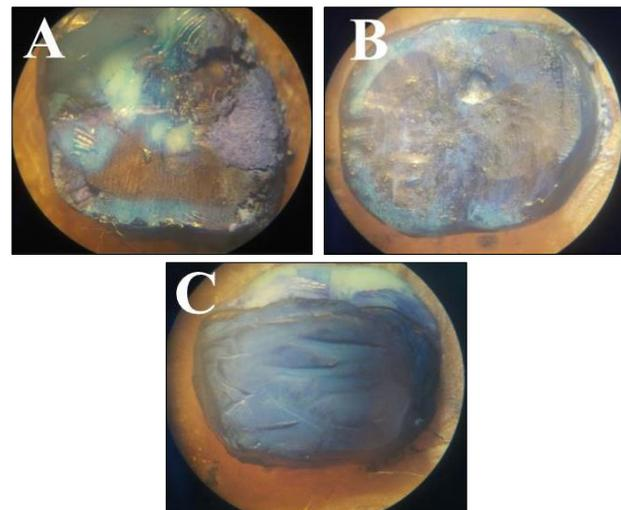
Figure 1: Failure modes as seen under stereomicroscope A) Mixed failure (B) Adhesive failure (C) Cohesive failure
